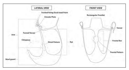
Figure 9. Structural scheme of type 1.B muzzles.
